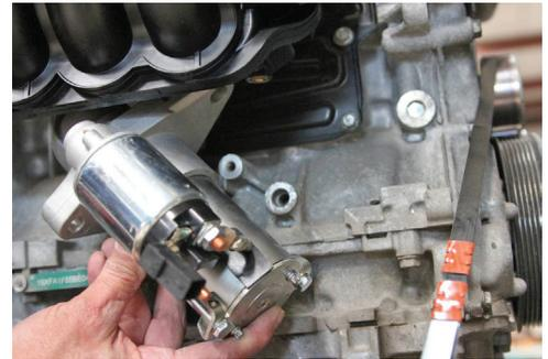
Figure 3: Raising the rear of the starter up and sliding the assembly to the bell housing.
