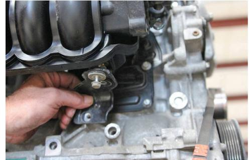
Figure 2: Rotating the starter nose to the 10 to 11 o'clock position.
