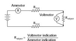
$$R_{\text{subject}} = \frac{\text{Voltmeter indication}}{\text{Ammeter indication}}$$
